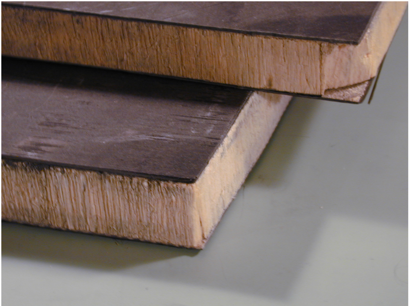
The famous bowling ball impact tests Pre-preg carbon skins over SuperLite Balsa Core
