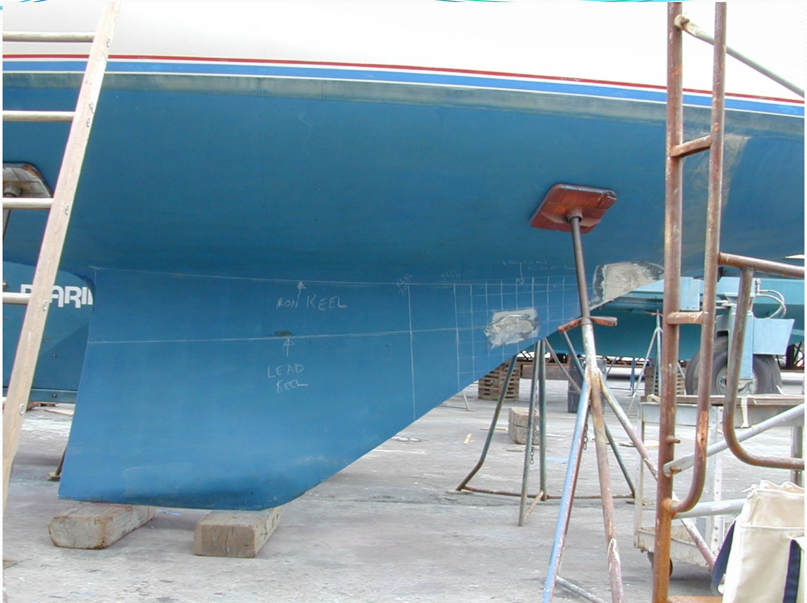
LEAD KEEL HAS LOWER C.G., MORE R.M.
