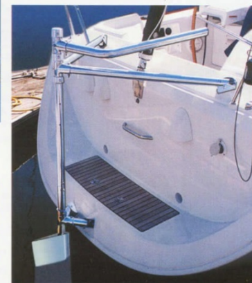
SOS Rudder installation on a Beneteau 42
