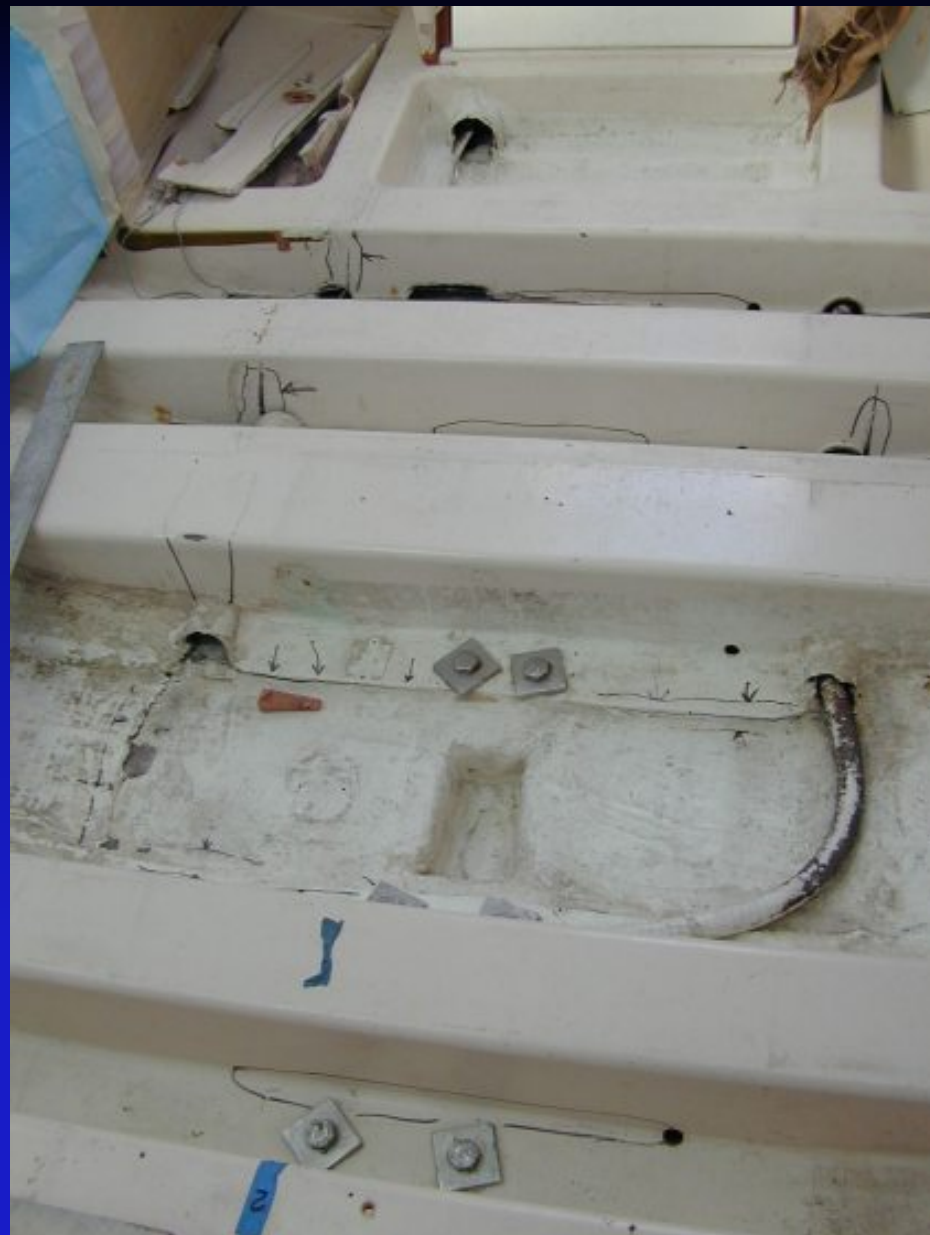
Grounding damage (two different boats)
