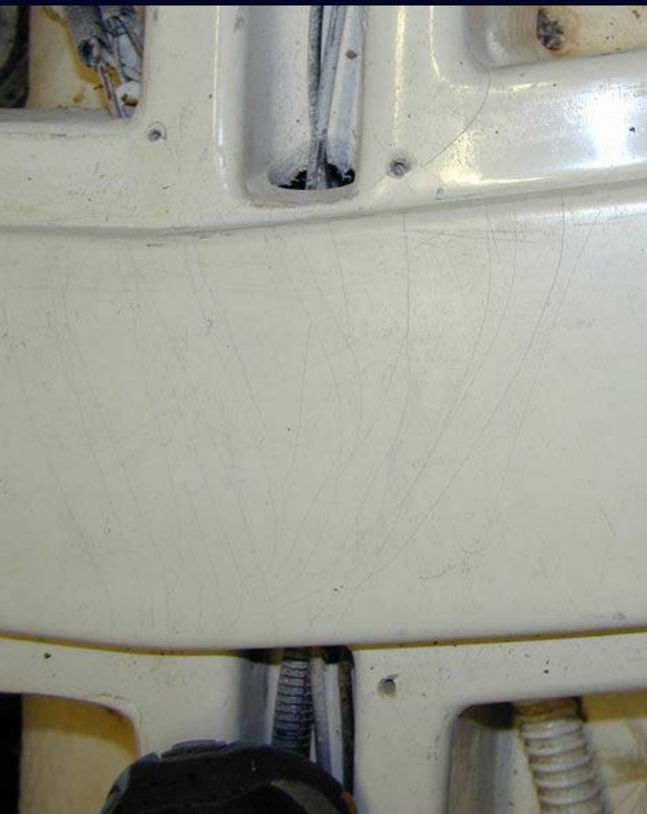
Grounding damage (two different boats)
