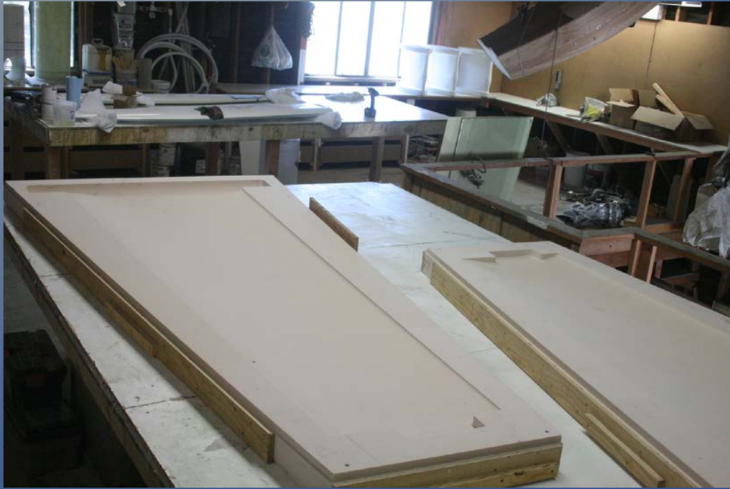
CNC cut keel fin molds Rudder blades in background
